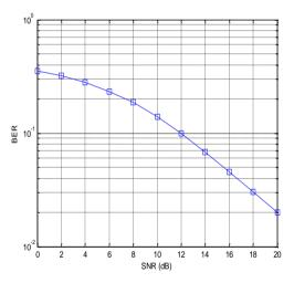
Fig 2. BER vs SNR performance of channel inversion precoding
