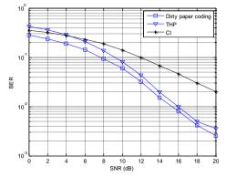
Fig 5. Comparison between the BER performance of CI, DPC and THP
