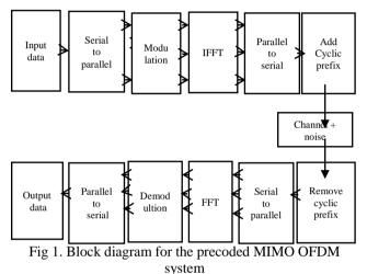
Data is the transmitted serially through the channels. At the receiver section the cyclic prefix is removed and Fourier transform is performed to obtain the frequency domain signals [10]. The demodulation is performed and the output data is obtained at the receiver end.
