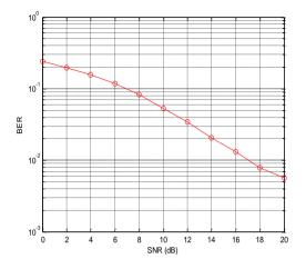
Fig 3. BER performance of Block Diagonalization precoding
