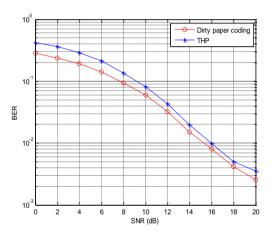
Fig 4. BER vs SNR plot of DPC and THP
